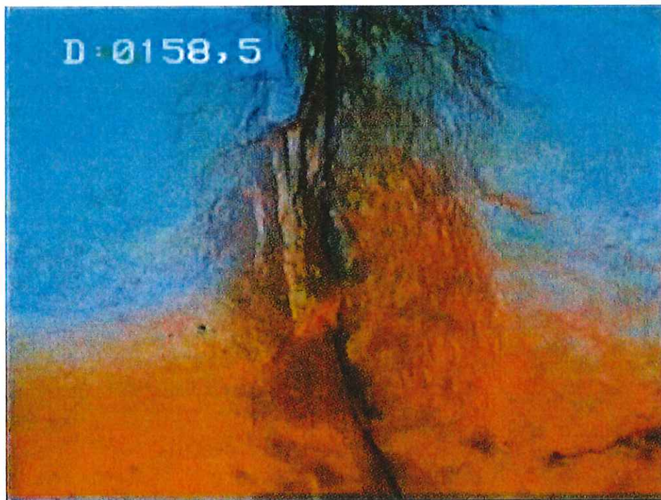
42- Trou nu – formation carbonatée massive, fracturation verticale
